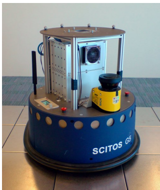
Figure 3: Swilly , THE METRALABS SCITOS G5 MOBILE ROBOT USED IN THE EXPERIMENTS
